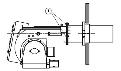
1. Remove 3 bolts connecting the burner body to the flame tube
