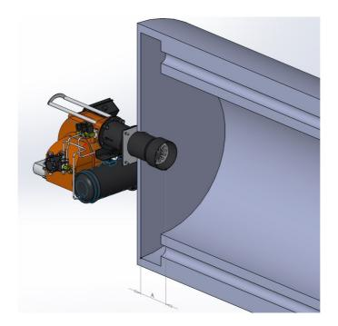
While installing the burner in reverse flame front mirror boilers, flame tube tip must be adjusted such that it gets inside by 50 mm-100 mm from flue pipes ( $50mm \le A \le 100mm$ ). Otherwise flue gas temperature will rise and fuel consumption will increase.
