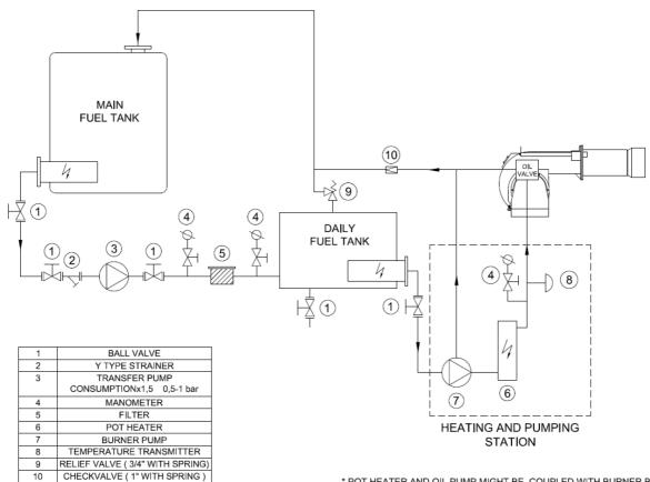
\* POT HEATER AND OIL PUMP MIGHT BE COUPLED WITH BURNER BODY OR COME AS A SEPARATE FILTERING-PUMPING-HEATING GROUP ACCORDING TO BURNER CAPACITY.
