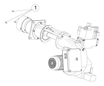
Remove 3 bolts number 1 that fix the body on the flame tube and pull back the body by sliding it on the lift shaft.
