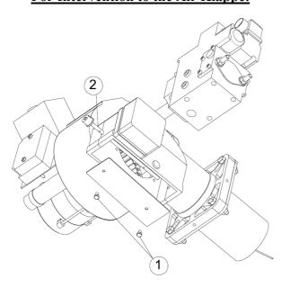
Remove 1 bolts number 2 that fix the klappe on the shaft. Detach the klappe and the shaft number 2 from the body.
