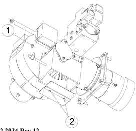
Remove the bolt number 1 from the shaft. Remove 2 bolts number 2 that fix the klappe on the shaft. Detach the klappe and the shaft from the body.
