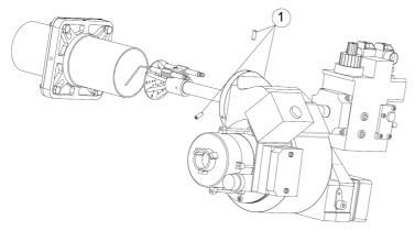
Remove 3 bolts number 1, which fix the flame tube on the Body, and pull back and lower the body provided that the flame tube stays on the boiler. Make the necessary intervention to ignition and ionization circuit.
