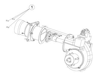
Remove 3 bolts number 1 that fix the body on the flame tube and pull back the body by sliding it on the lift shaft.
