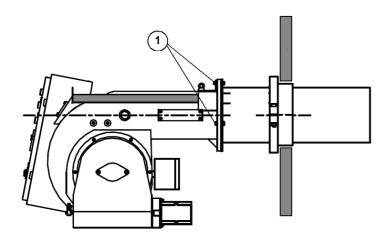
1. Remove 3 bolts connecting the burner body to the flame tube
