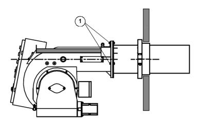
1. Remove 3 bolts connecting the burner body to the flame tube
