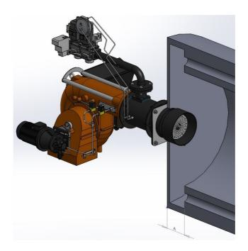
While installing the burner in reverse flame front mirror boilers, flame tube tip must be adjusted such that it gets inside by 50 mm-100 mm from flue pipes ( $50 \text{mm} \le A \le 100 \text{mm}$ ). Otherwise flue gas temperature will rise and fuel consumption will increase.
