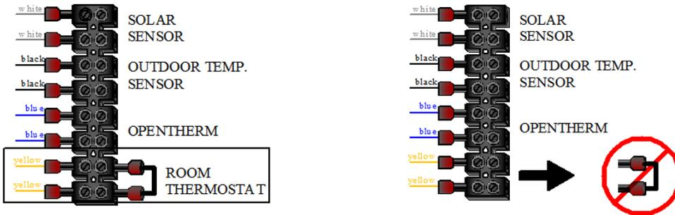
Closure of Room Thermostat contact generates a heat demand in CH mode.
