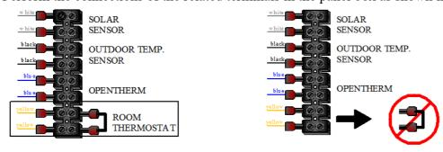
Closure of Room Thermostat contact generates a heat demand in CH mode.
