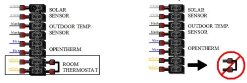
Closure of Room Thermostat contact generates a heat demand in CH mode.
