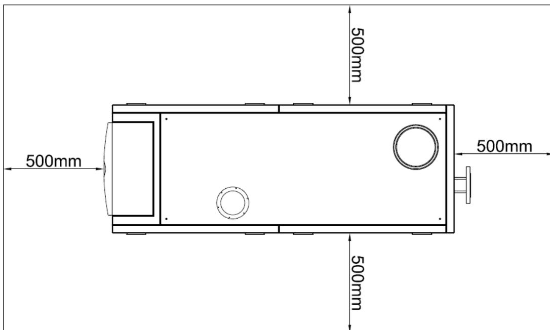
**i** There must be at least 500 mm of gap between adjacent boilers and at least 500 mm of space in front of the boiler for ease of service.
